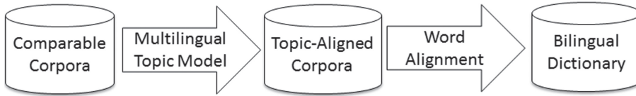
Fig. 1. The proposed framework for bilingual dictionary extraction. A multilingual topic model is used for converting a document-aligned comparable corpus to topic-aligned corpora. Given a topic, word alignment models are used to model co-occurrence across languages.
