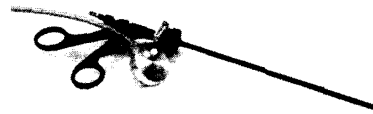
3. Instrument mounted joystick: The embodiment shown is the functional equivalent of a three button mouse.
