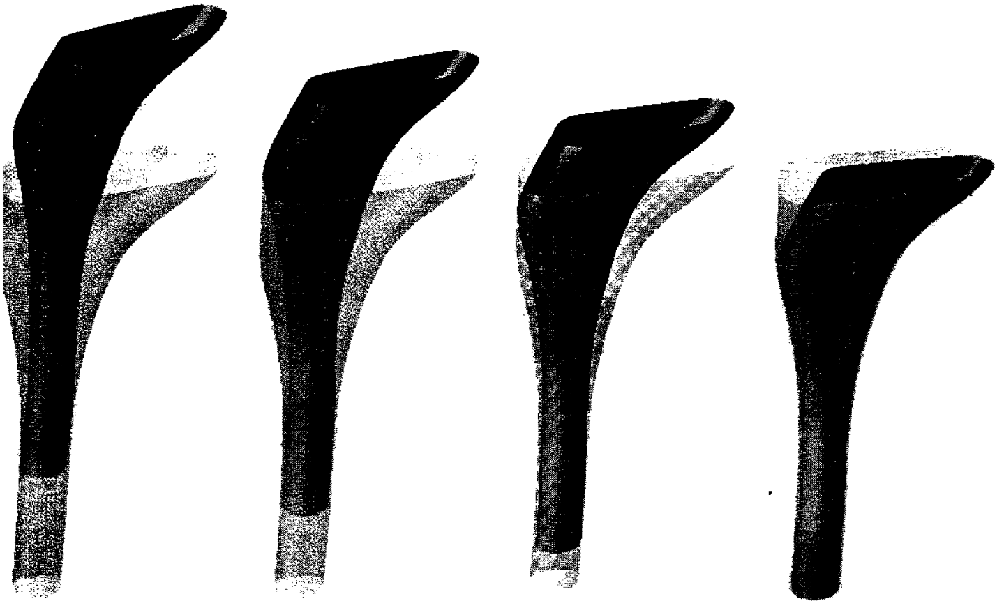
Fig. 3. Snapshots of an insertion sequence of an implant stem (dark body) into a canal (translucid body) from the initial (left) to the final (right) configuration.
