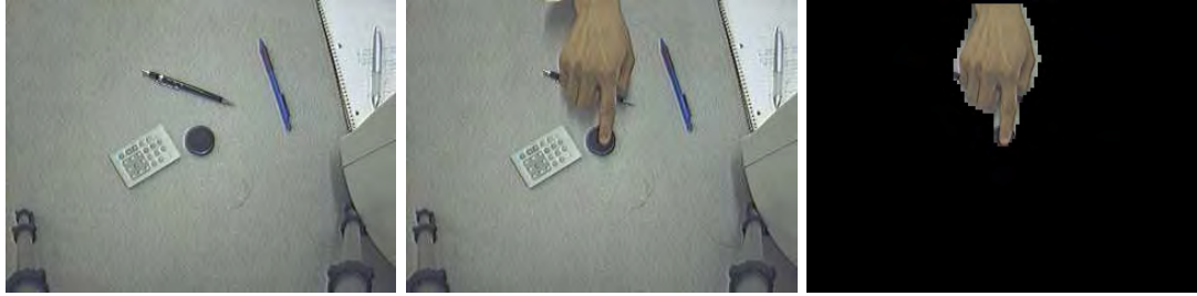
Figure 4.8: An example of background image, unsegmented image and segmentation result. The leftmost image is the background. The second image shows when the hand has entered the scene. The final segmentation result is shown in the third image.
