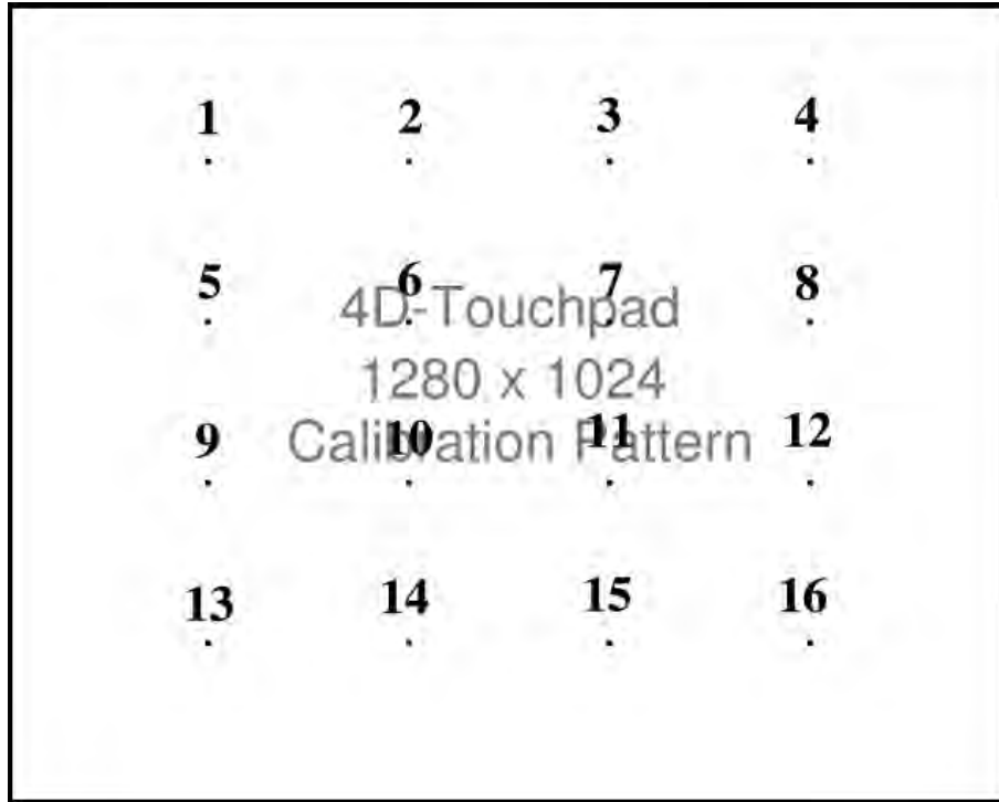
Figure 5.2: Calibrate pattern used in homography computation.
