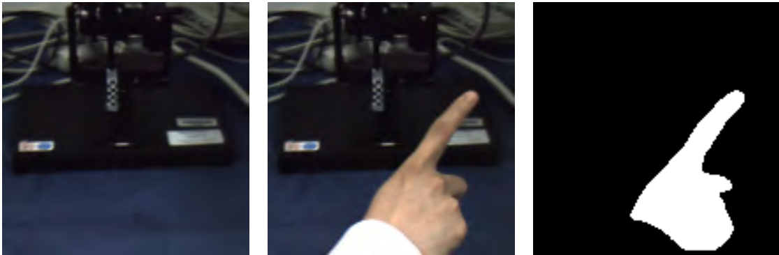
Figure 3.2: An example of background image (left), foreground image (middle) and segmentation result (right).
