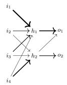
Fig. 1: A small acyclic neural network. The activation  $x_n$  at each node n is a nonlinear function f, such as a sigmoid or threshold function, of a weighted sum of activations at n's parent nodes:  $x_n \stackrel{\text{def}}{=} f\left(\sum_{(n',n)\in E} x_{n'}w_{n',n}\right)$ . The three layers shown here are the traditional input, hidden, and output nodes, with  $w_{n',n}$  values represented by arrow thickness.
