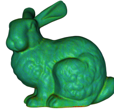
Fig. 2: An analysis of correctness: A comparison of several different reconstructions of the Bunny dataset at depth d = 9 created with the distributed implementation. The table summarizes the size of each model, and the maximum and the average distance of each vertex from the ground-truth. The image on the right shows the distribution of error across the p = 8 model. The color is used to show \delta values over the surface with \delta = 0.0 colored blue and \delta = 1.0 colored red.
