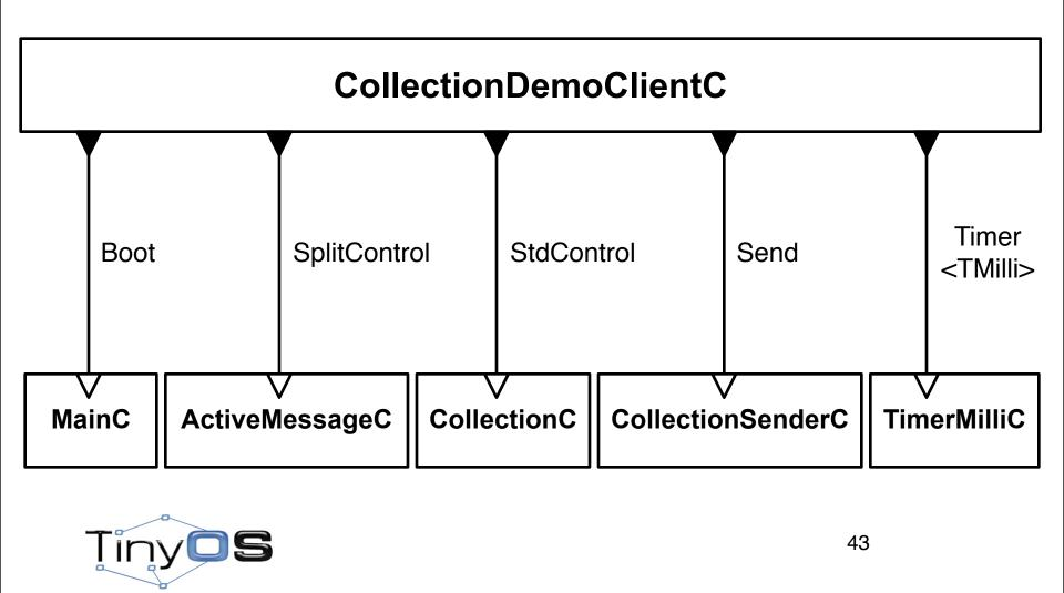
This is the components and interfaces we need. The CollectionC is component that offers the StdControl interface for collection. The CollectionSenderC is the offering a Send interface to send the value up on the tree.
