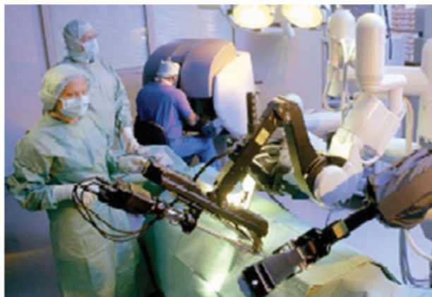
Fig. 3. The da Vinci surgical robot uses mechanically constrained remote-center-of-motion arms manipulate modular tools under surgeon teleoperator control. The tools use cable drives to provide high-dexterity manipulation inside the body. (Photo: Intuitive Surgical Systems).
