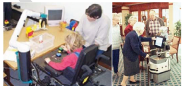
Fig. 14. Robots for assistance in daily living. Left: exact dynamics assistive robot manipulator [49]. Right: CMU Nursebot [49].
