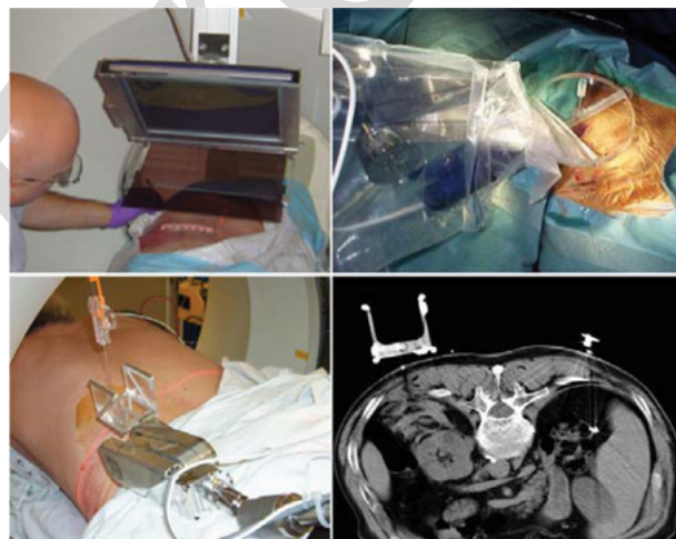
Fig. 12. Needle placement under image guidance. Top left: in-CT freehand placement with image overlay device [110]. Top right: x-ray guided nephrostomy needle placement [81]–[83]. Bottom: in-CT kidney biopsy with fiducial structure on needle driver to assist robot-to-scanner registration [111], [112].
