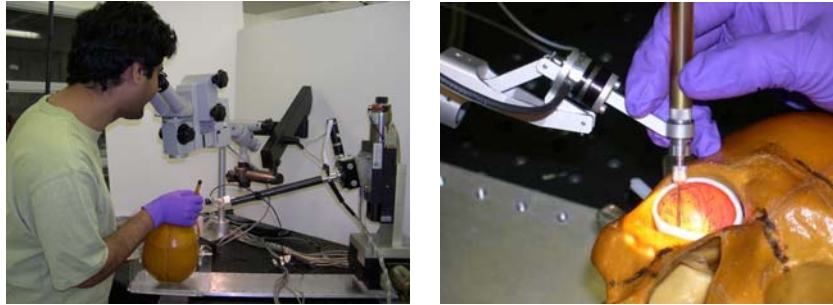
Fig. 4. The new steady-hand manipulator for retinal surgery.
