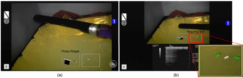
Fig. 4. (a) The graphical probe widget indicates the transducer and image orientation as well as wrist configuration. (b) A mapping tool indicates the current probe position and orientation (white cursor), as well as “bread crumbs” (green markers).
