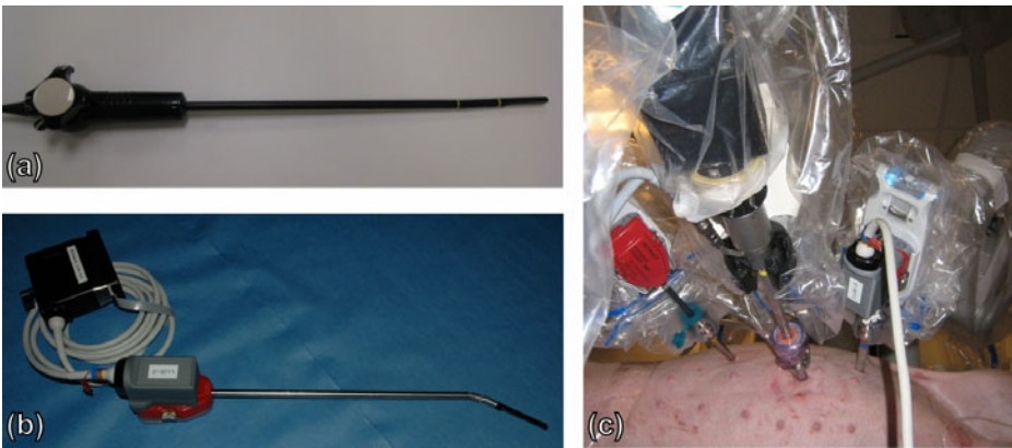
Fig. 2. (a) A hand-held laparoscopic ultrasound probe (Aloka UST-5536-7.5). (b) The prototype da Vinci ultrasound instrument. (c) The ultrasound instrument manipulated by a da Vinci robotic manipulator.
