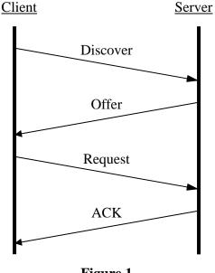
**Figure 1** DHCP Four-way handshake
