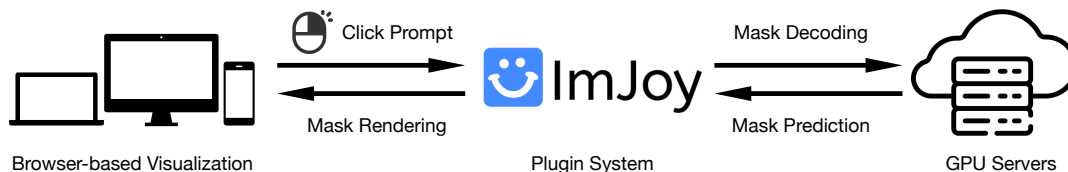
Figure 1: The diagram of our interactive segmentation tool.
