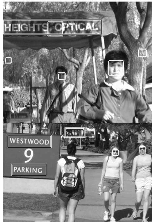
Figure 6: The boxes show faces and text as detected by AdaBoost. Observe the false positives due to vegetation, tree structure, and random image patterns. It is impossible to select a threshold which has no false positives and false negatives for this image. Instead we use AdaBoost to output conditional probabilities, which will take their biggest values in the boxes, which are used in the DDMCMC algorithm.
