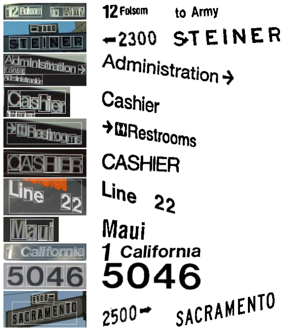
Figure 9: Extension (left column) and binarization of the text regions shown in figure (8). Note that our OCR software is not yet able to read Chinese or Spanish so we treat these as non-text.
