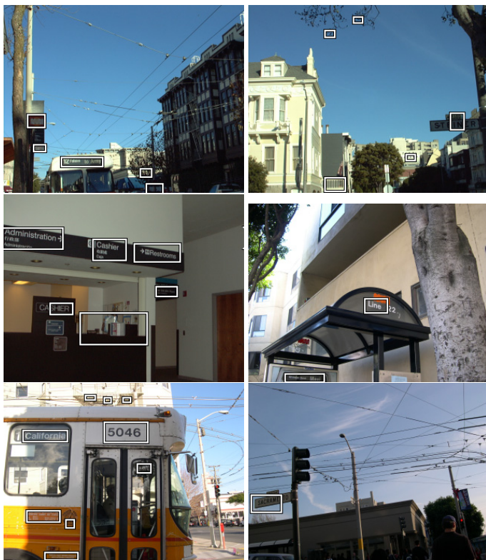
Figure 8: Results of AdaBoost on typical test images (taken by blind subjects). The boxes display areas that AdaBoost classifies as text. Observe that text is detected at a range of scales and at non-horizontal orientations. Note the small number of false positives. The boxes will be expanded and binarized in the next processing stage.
