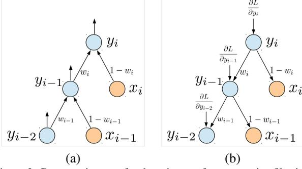
Figure 3. Computation tree for domain transform recursive filtering: (a) Forward pass. Upward arrows from  $y_i$  nodes denote feeds to subsequent layers. (b) Backward pass, including contributions  $\frac{\partial L}{\partial y_i}$  from subsequent layers.
