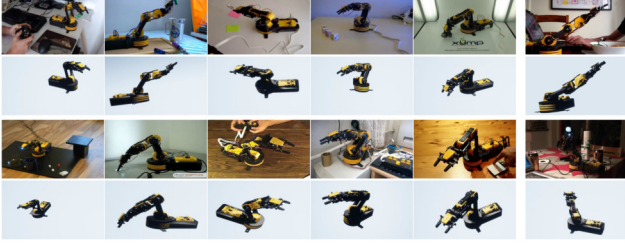
Figure 5. Qualitative results from our YouTube dataset. The challenges include occlusion, user modification, lighting, etc. We show synthetic images generated using the camera parameters and pose estimated from the single input image. Both success cases (left five columns) and failure cases (rightmost column) are shown.
