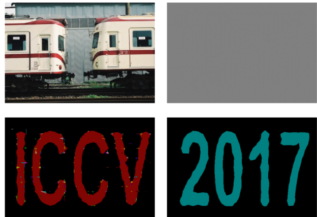
Fig. 4 Figure taken from Xie et al. (2017). The top row is the input (adversarial perturbation already added) to the segmentation network, and the bottom row is the output. The red, blue and black regions are predicted as airplane , bus and background , respectively.
