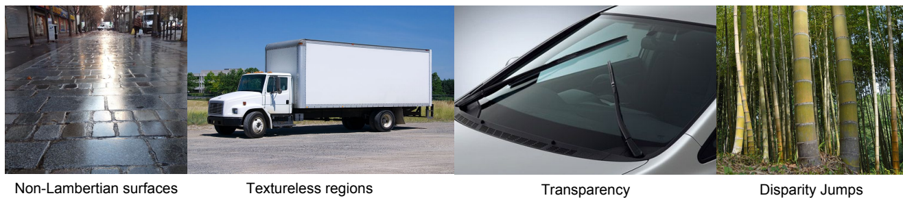
Fig. 6 Hazardous factors for stereo vision, as identified in Zendel et al. (2015). These challenging scenarios may not occur in real world datasets, and if they do they are not annotated, so relying on synthetic data is a promising alternative.
