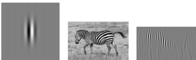
Fig. 16. A Gabor functions aligned to the vertical axis (left). The image of a zebra (center). The response of the vertical Gabor filter on the zebra image (right).
