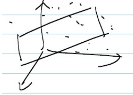
Figure 5: PCA can be obtained as the projection which minimizes the least square error of the residuals.
