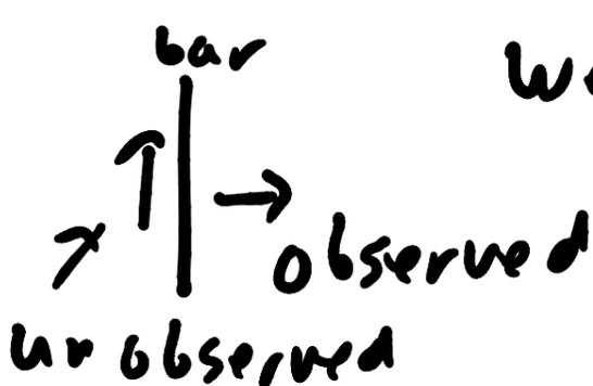
We can observe the motion in the direction perpendicular to the bar. But we cannot observe the motion along the bar.
