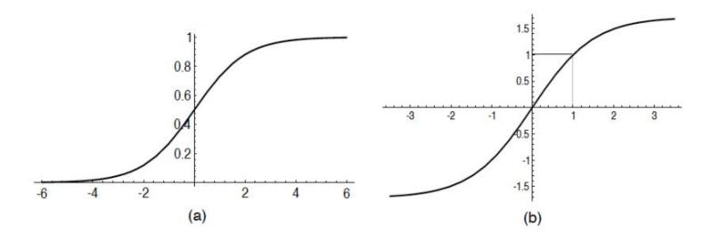
**Fig. 4.** (a) Not recommended: the standard logistic function,  $f(x) = 1/(1 + e^{-x})$ . (b) Hyperbolic tangent,  $f(x) = 1.7159 \tanh\left(\frac{2}{3}x\right)$ .
