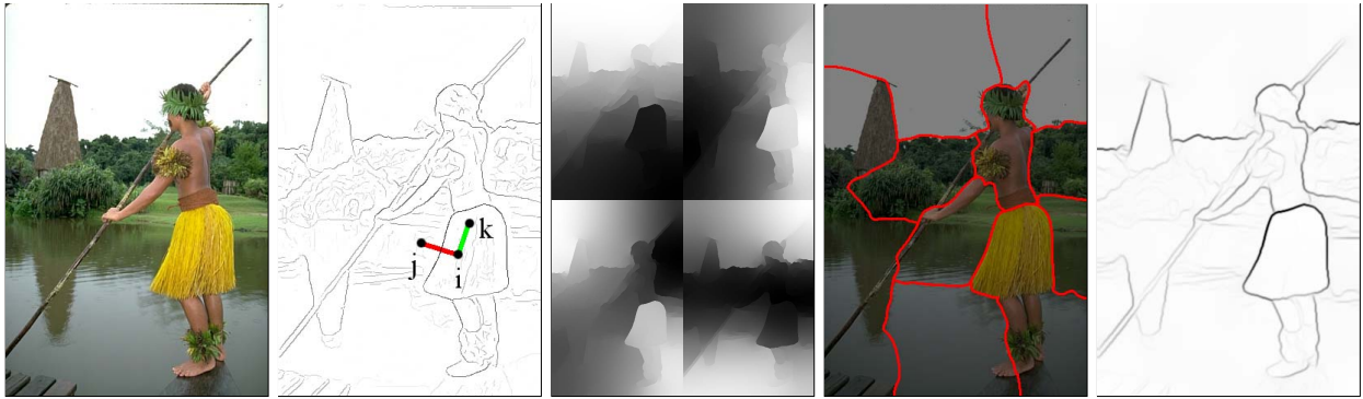
Figure 6: Spectral Pb. Left: Image. Middle Left: The thinned non-max suppressed multiscale Pb signal defines a sparse affinity matrix connecting pixels within a fixed radius. Pixels i and j have a low affinity as a strong boundary separates them, whereas i and k have high affinity. Middle: First four generalized eigenvectors resulting from spectral clustering. Middle Right: Partitioning the image by running K-means clustering on the eigenvectors erroneously breaks smooth regions. Right: Instead, we compute gradients of the eigenvectors, transforming them back into a contour signal.
