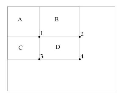
Using the integral image representation one can compute the value of any rectangular sum in constant time.
