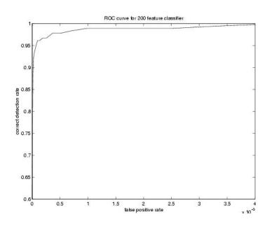
The ROC curve of the constructed classifies indicates that a reasonable detection rate of 0.95 can be achieved while maintaining an extremely low false positive rate of approximately  $10^{-4}$ .
