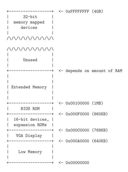
The first PCs, which were based on the 16-bit Intel 8088 processor, were only capable of addressing 1MB of physical memory. The physical address space of an early PC would therefore start at 0x00000000 but end at 0x000FFFFF instead of 0xFFFFFFFF. The 640KB area marked "Low Memory" was the only random-access memory (RAM) that an early PC could use; in fact the very earliest PCs only could be configured with 16KB, 32KB, or 64KB of RAM!
