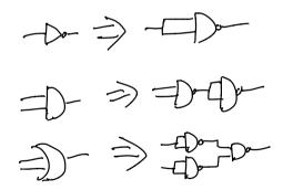
So given circuit  $\boldsymbol{C}$ , first transform it into NAND-only circuit.
