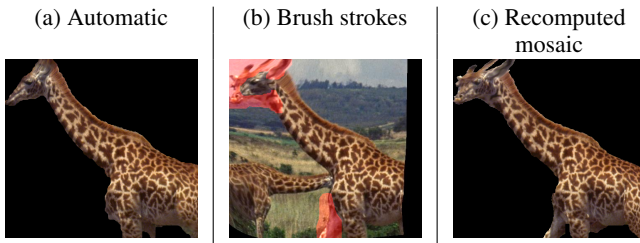
Figure 8: User interaction. (a) Automatically computed mosaic for giraffe sequence. The far side of the head, and the distal leg, are not represented as they appear in too few frames. (b) User brush strokes on an intermediate frame inverse-warped into parameter space. The strokes indicate parts of this frame which should appear in the mosaic. (c) New mosaic computed with only the brush strokes in (b) as constraints. The head and leg are now present in the mosaic, so can be matched to the original sequence during mapping refinement.
