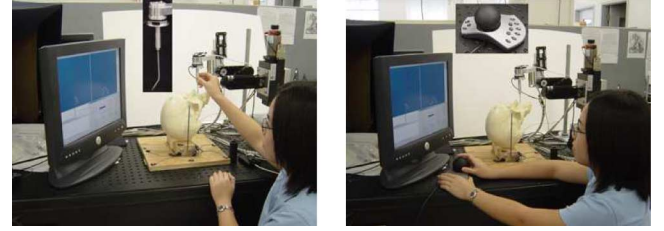
Fig. 10. (left) Hands-on cooperative control. (right) Teleoperative control. In hands-on cooperative control, a force sensor and tool are mounted on the robot end-effector. Tool is manipulated by an operator holding a handle attached to the force sensor. The robot read the applied force and provided assistance. In remote teleoperative control, we used a 3-D mouse to telecontrol the robot.
